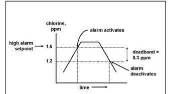
**FIGURE 5-1. High alarm logic.** The alarm activates when the chlorine concentration exceeds the high setpoint. The alarm remains activated until the reading drops below the value determined by the deadband.
